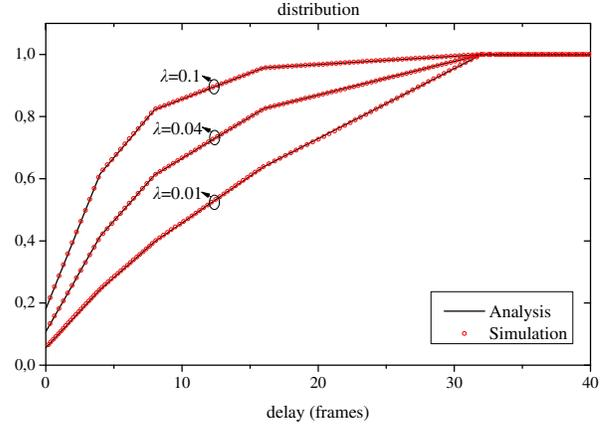
Fig. 2. Distribution of the type-I sleep mode delay. Settings:  $s_{\text{min}} = 4$ ,  $s_{\text{max}} = 32$ ,  $l_{\text{init}} = 2$ ,  $l = 1$  and  $\lambda = 0.01, 0.04, 0.1$ .
