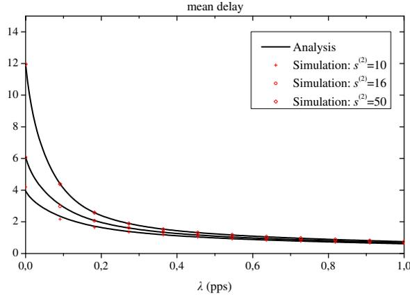
Fig. 4. Multiclass mean delay as a function of the arrival rate. Settings:  $m = 4$ ,  $s_{\min} = 4$ ,  $s_{\max} = 32$ ,  $l_{\text{init}} = 2$  and  $l = 1$ .
