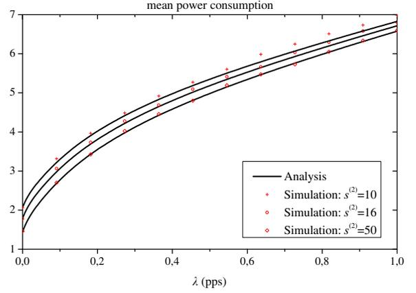
Fig. 5. Multiclass mean power consumption as a function of the arrival rate. Settings:  $P_L = 10$ ,  $P_S = 1$ ,  $m = 4$ ,  $s_{\min} = 4$ ,  $s_{\max} = 32$ ,  $l_{\text{init}} = 2$  and  $l = 1$ .
