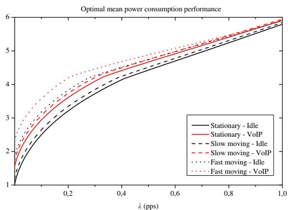
Fig. 7. Mean power consumption with QoS guarantees for delay in several application scenarios. Settings:  $P_L = 10$ ,  $P_S = 1$ ,  $l_{init} = 2$ ,  $l = 1$ ,  $d_{thr} = 5$ ,  $\alpha = 0.95$ , for slow moving  $s^{(2)} = 50$ , for fast moving  $s^{(2)} = 10$  and for VoIP  $s^{(2)} = 16$ .
