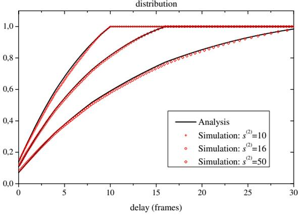
Fig. 3. Distribution of the multiclass sleep mode delay. Settings:  $s_{\min} = 4$ ,  $s_{\max} = 32$ ,  $l_{\text{init}} = 2$ ,  $l = 2$  and  $\lambda = 0.01$ .
